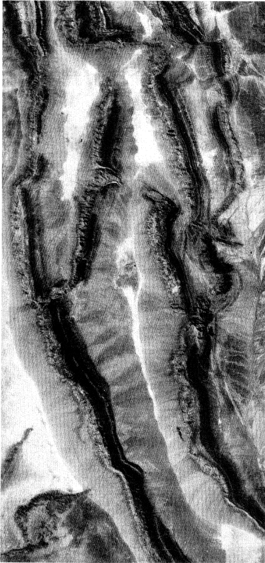
FIGURE 11. Landsat mss band 7 image over Kelpin Tagh, western Sinkiang, China. Landsat path/row 159/32, 15 May 1973, centre point N 40° 25', E 78° 17'. Sun elevation 59° from southeast (top left-hand corner). The better resolution and depiction of surface roughness of the SIR-A results in better definition compared with Landsat.
