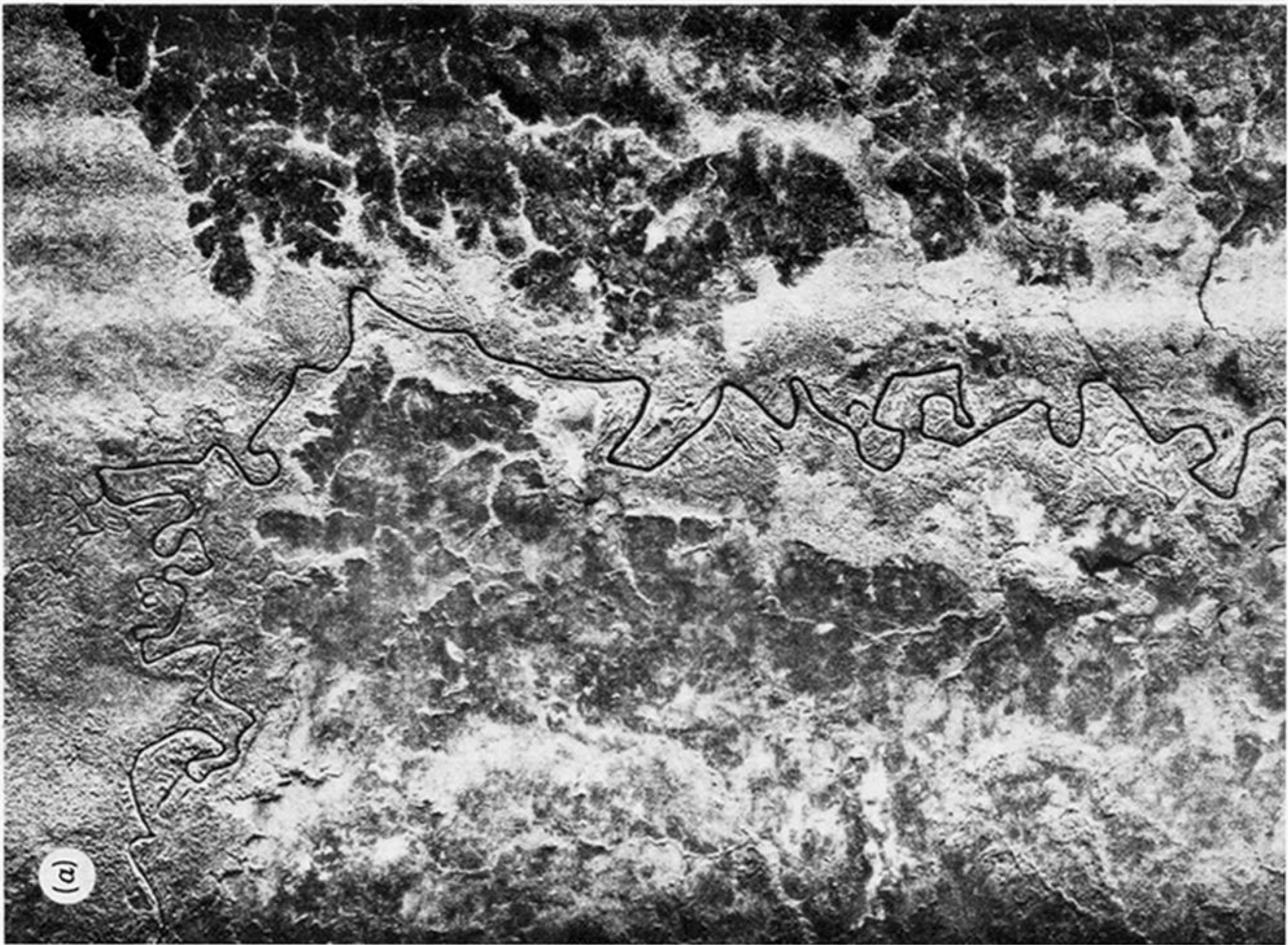
FIGURE 12. Comparison of (a) Westinghouse Ka (0.86 cm) SLAR and (b) L-band (23 cm), SIR-A (data-take 24C) over low-relief area of northeast Nicaragua. Scale nominally 1:200 000. Area of forest and cleared forest savanna underlain by clays and gravels. Although the SIR-A has distinctly inferior resolution (40 m compared with 10 m) laterite-surfaced roads can show well. Differences of tone on the imagery are thought to be due to temporal changes (the two images are 10 years apart, but both of wet season) rather than radar wavelength differences. The dark interfluvial areas are probably waterlogged savannah. The radar illumination is from the right-hand side of the image for the SLAR, at an incidence angle of ca. 60°; that for the SIR-A is from the top left-hand corner of the image at an incidence angle of 50°. Note that the marked difference of radar illumination and depression angle do not materially change the delineation of radar geological units.
