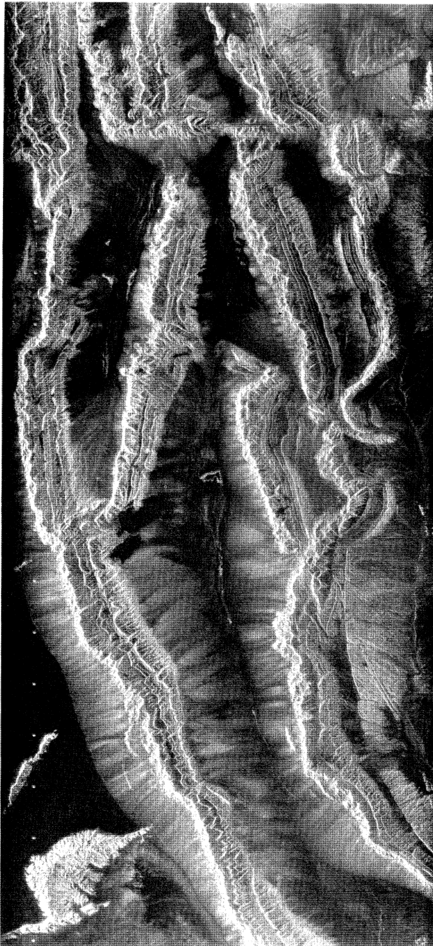
FIGURE 10. SIR-A image (data-take 28) over Kelpin Tagh, western Sinkiang, China, between Tien Shan ranges and Takla Makan desert. Scale approximately 1:500 000. In this arid area folded and thrust sedimentary rocks are cut by prominent transcurrent faults. Thrust planes dip northward (towards bottom of image). Large cuestas are surrounded by alluvial fans whose rough cobble and boulder surfaces provoke a bright radar response. The boundary between fans and desert sands, which have almost no radar backscatter, is distinct (top left of image). Radar illumination from top of image at approximately 50^\circ incidence angle; north is approximately to bottom left of image. The white dots are fiducial marks representing each second of the Shuttle's orbit.
