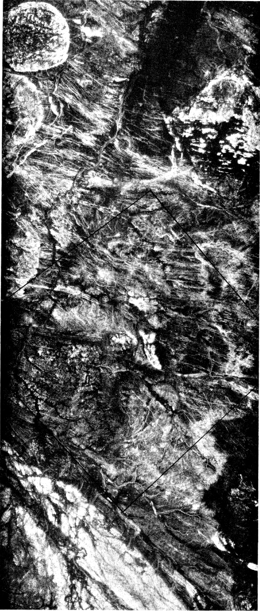
FIGURE 8. SIR-A swath 29/30 over Adrar des Iforas, northeast Mali. Scale nominally 1:500 000. Bright areas are rough-surfaced outcropping rock; black tonal areas are thick sand. 'Younger Granite' ring-intrusions and associated dyke-swarms and the Iforas granulite unit are particularly distinct. The radar illumination is from top of image, north is to bottom left corner. The area of the subscene in figure 9 b is shown. The margins are not rectangular because the subscene has been 'warped', on an image processor, to co-register with Landsat.
