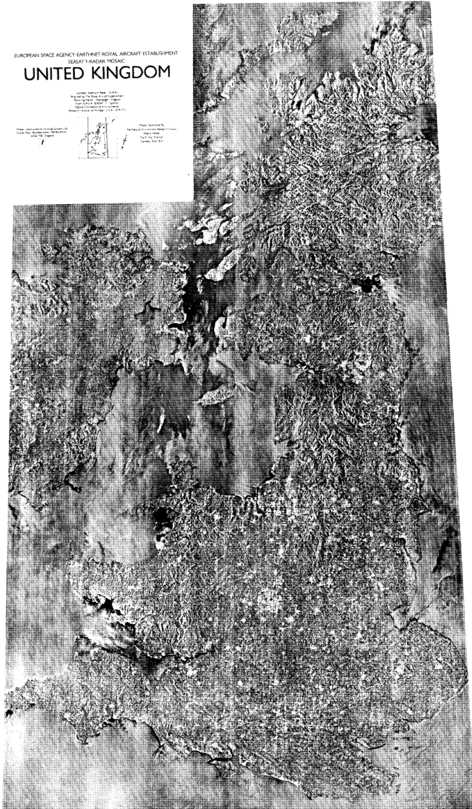
FIGURE 3. Seasat radar mosaic of the United Kingdom and adjacent Ireland, constructed by Hunting Surveys Limited for the R.A.E./E.S.A.-Earthnet and N.E.R.C. (N.A.S.A.'s Seasat 1 SAR data acquired at R.A.E. Oakhanger and optically correlated by E.R.I.M., U.S.A.).
